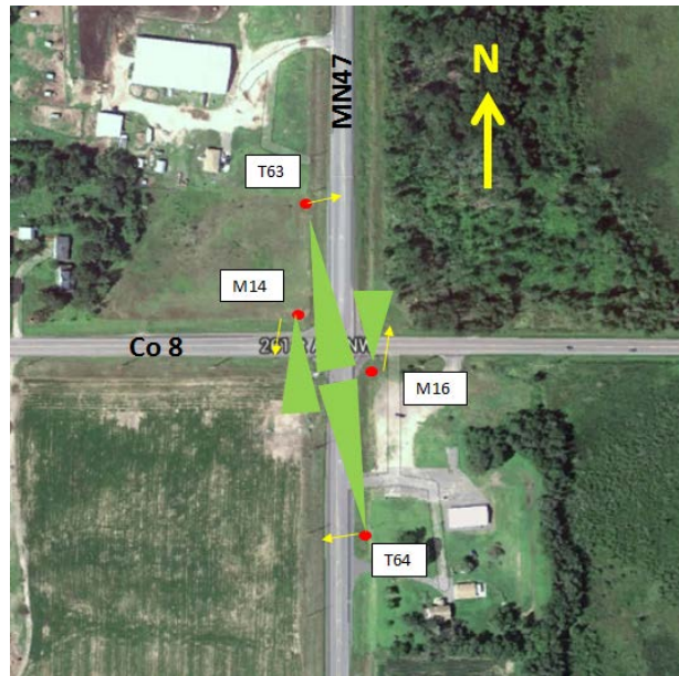
Figure 7: Isanti treatment intersection camera layout
